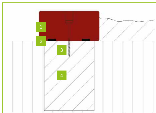
1 Regupol® Sandpit Safety Surrounds • 2 Gluing • 3 Screw connection/fixing with dowels • 4 Concrete base
